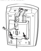
7. Plug the short modular cord's other end into the wall plate jack, align the base's keyhole slots with the wall plate studs, and slide the base downward to secure it.
